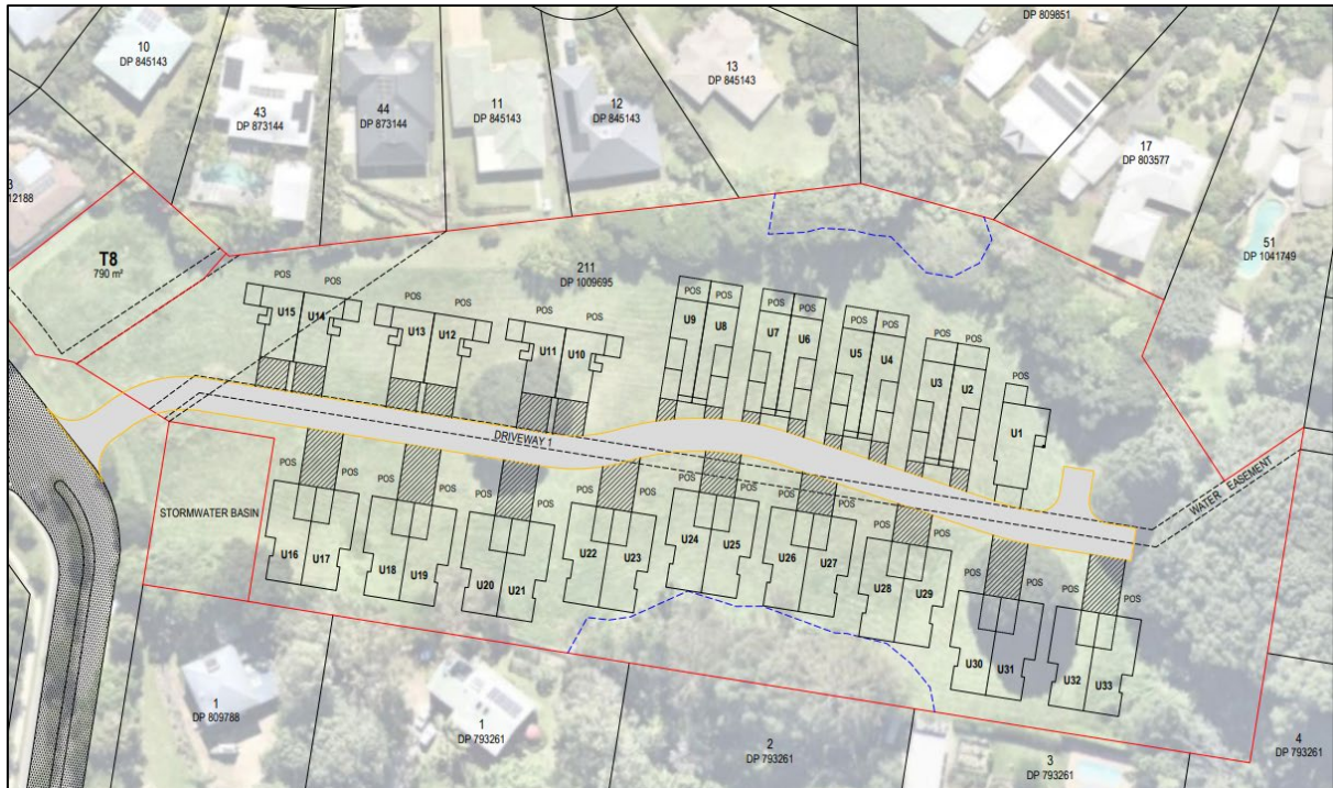
Figure 12: Eastern precinct - Approximate 9m APZ setback distance from hazard vegetation on-site and stormwater basin, subject to confirmation of permitted tree removal. Potential to reduce the APZ with performance solutions.
