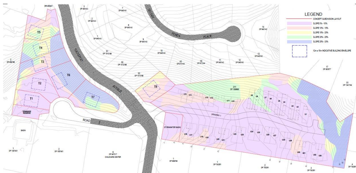
Figure 13: Slope Analysis Plan (Civiltech Consulting Engineer)
